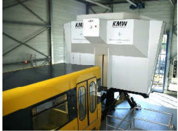
Figure 1 and 2: Full cabin simulators (1. generation): BVG-Tram (left), SSB-AG Stadtbahn (right), view presentation via projection, 6 DOF electromechanical moving system
